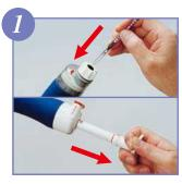
Insert <u>a sealed</u>, <u>unbroken detector</u> <u>tube</u> into the rubber tube connector. Align the red line on the bottom case and that of shaft, and pull the handle to full stroke locked position.
